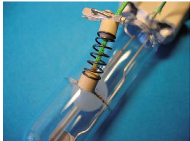
Fig. 35: Clamping the thermocouple on the outer bulb using a spring element
