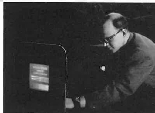
Fig. 4. A demonstration of a method of amplifying light. The equipment is a single plate image converter (shown by BTH) using cadmium sulphate crystals.
