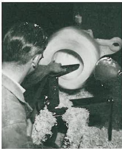
▲ A Satina shade takes shape. This mould maker was trained by a German who joined Hailwood & Ackroyd in 1920 and believes that there are only two other men in his trade in Britain. Moulds cut from wet sappy beechwood or pear wood take about three days to make. They form their own layer of charcoal in use giving glass with a very high quality finish. A similar iron mould might take six weeks to prepare. The wooden hand tools used by the blowers in shaping the glass are also made in this department.
