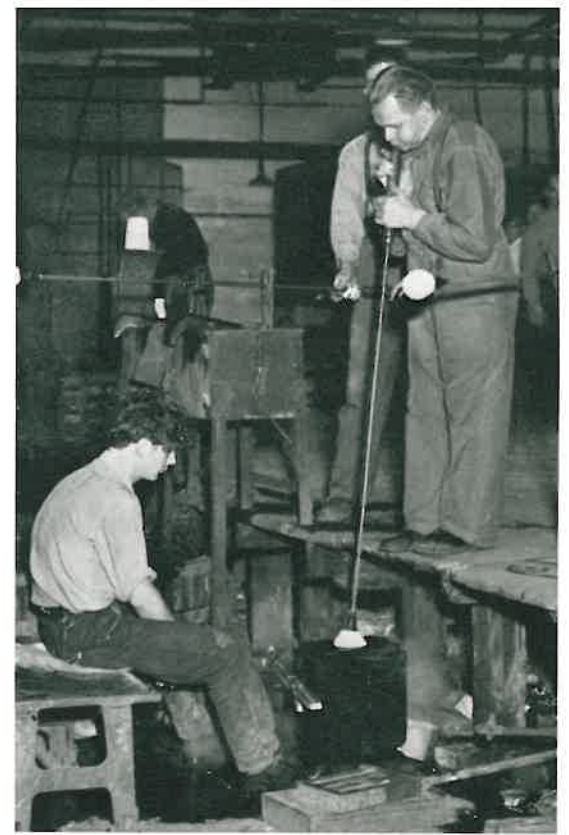
▲ A craftsman puts the finishing touches to the blowing of a shade while rotating in a wet mould. The surface of the glass is formed against the charcoaled wood of the mould and a cushion of steam. The two other balls of glass in the picture are in the hands of the ball blowers who will pass them to the glass blower to be finished.
