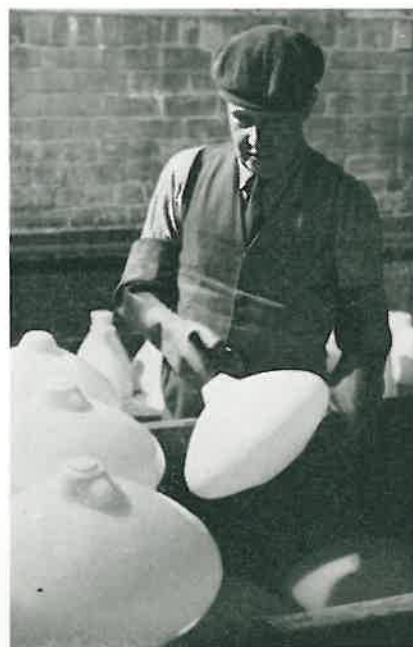
▲ Satin etching puts the final touch to the glass. Notice the difference in appearance between the etched shade and the others which have yet to be put into the acid bath.
