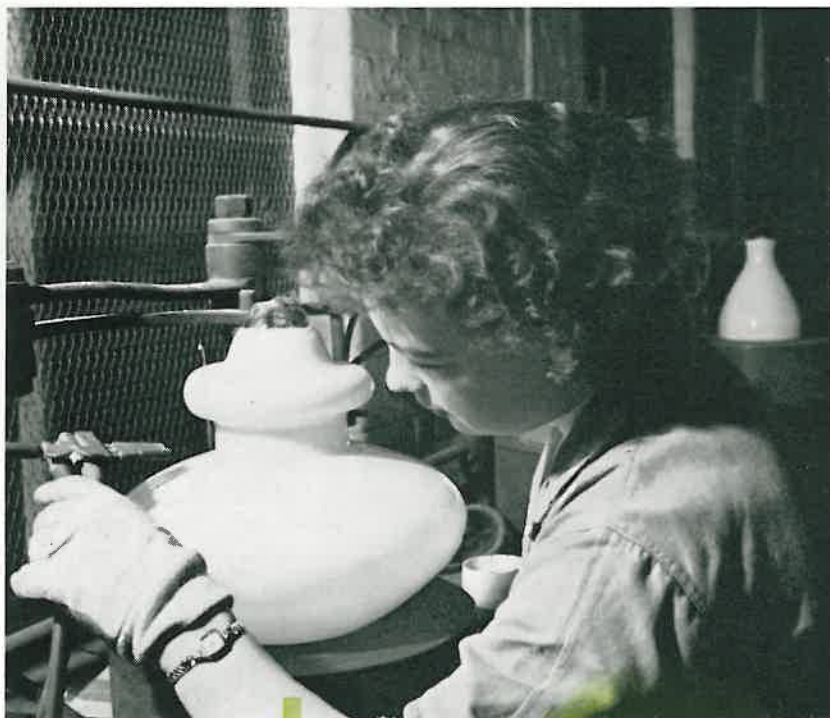
▲ After annealing, surplus glass is trimmed from the shade by localized heating with gas jets followed by a scratch with a diamond (below) and then cut edges are ground on revolving steel plates with carborundum powder and water. (Second colour illustration below) ▼
