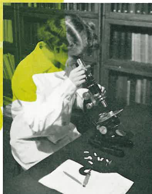
▲ A routine laboratory check on three-ply glass to ensure that no strain has been set up between the layers of opal and clear glass. ▼
