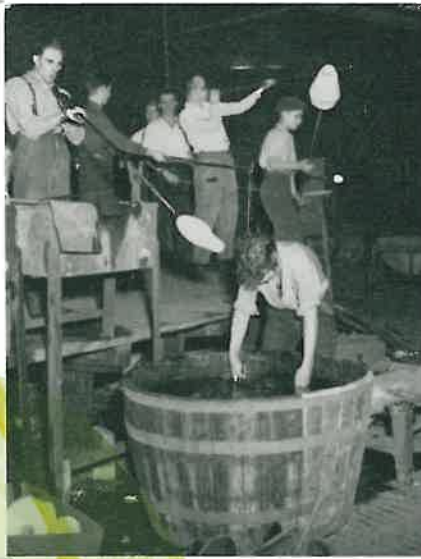
▲ Molten glass is gathered on blow-pipes at the furnace and blown and hand shaped with pear wood 'blocks' and 'pointers' before being finally shaped while rotating in a wet wooden mould. It is on preliminary shaping of the molten glass that the uniformity of thickness of the finished glass depends.
