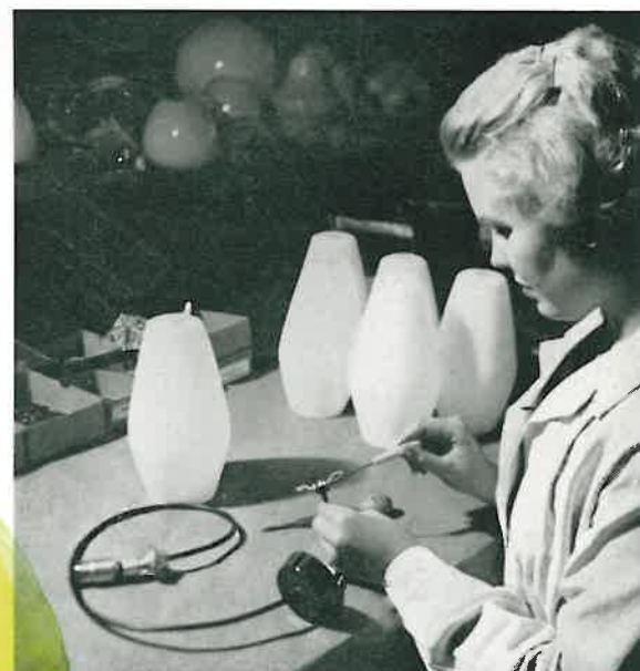
▲ Assembling a ceiling plate component for a single shade pendant. The anodized matt black cover plate is held in position by a sliding rubber grommet on the flex. ▼
