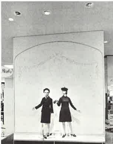
Three 250-watt PAR-38 Quartzline spots produce twice the illumination on mannequins—compared to regular 150-watt R-40's used previously.
