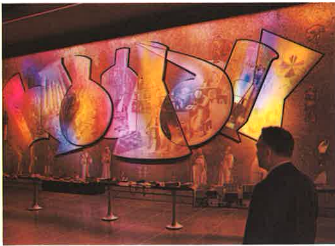
Here, the colored light comes from the front of the mural. PAR lamps with colored filters are closely spaced behind the dropped ceiling and aimed at Jon Bel-Jon's stainless steel creation. Designs are made with engraver's tools, and reflect different colors when they are viewed from different locations in the lobby.
