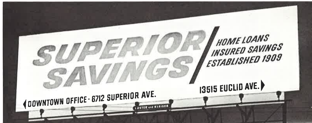
This painted bulletin measures about 20 feet by 60 feet. It is lighted by nine 1000-watt R-60 Quartzline floods. Lighting level is about 100 footcandles.
