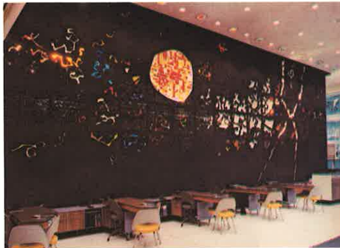
Here, the colored light comes from the front of the mural. PAR lamps with colored filters are closely spaced behind the dropped ceiling and aimed at Jon Bel-Jon's stainless steel creation. Designs are made with engraver's tools, and reflect different colors when they are viewed from different locations in the lobby.
