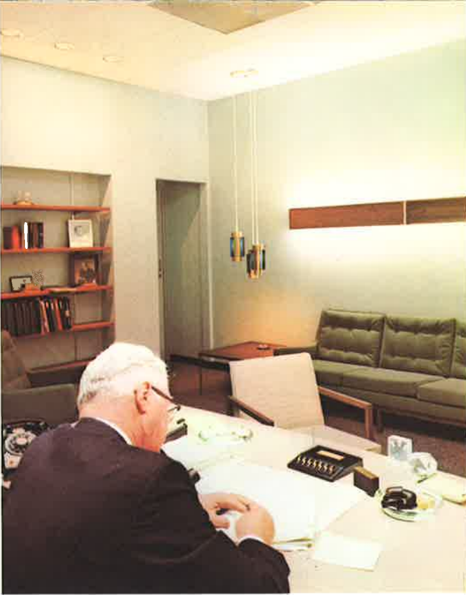
EXTENSIVE USE OF WALL LIGHTING. Walls occupy the greatest part of the visual field. Lighted walls can make a room look larger, can emphasize windows and artwork, and can help make up for a drop-off in lighting levels near the perimeter of a room . . . as it does in the private office, here.
