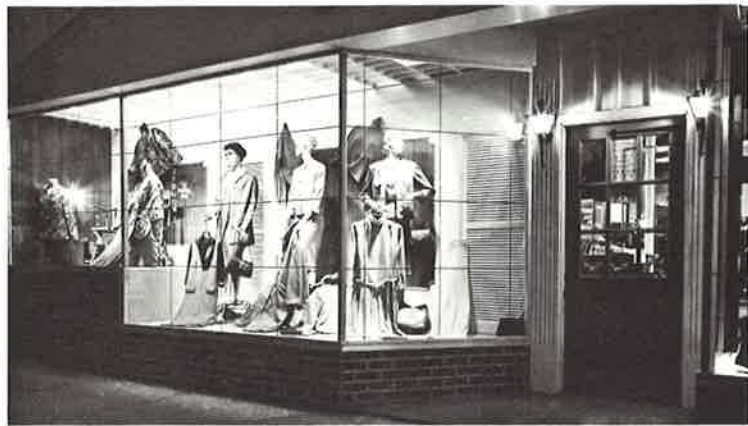
In this show window (close-up, left) are seven 250-watt PAR-38 Quartz-line floodlamps. These accent the merchandise — direct attention to it.
