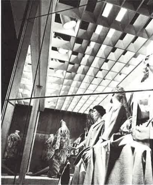
In this show window (close-up, left) are seven 250-watt PAR-38 Quartz-line floodlamps. These accent the merchandise — direct attention to it.
