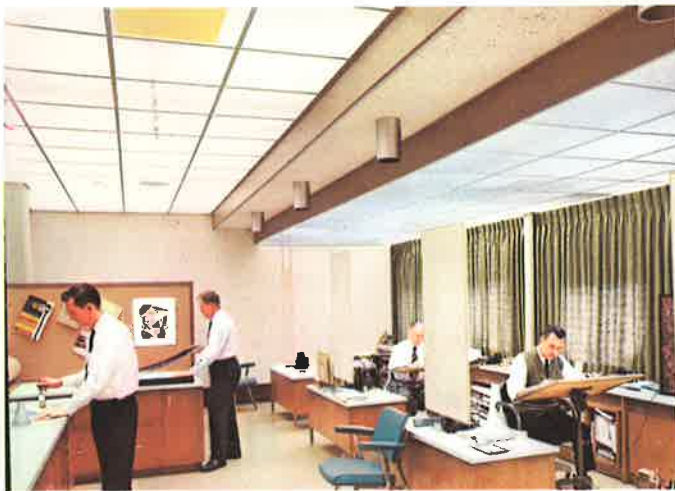
EXTENSIVE USE OF WALL LIGHTING. Walls occupy the greatest part of the visual field. Lighted walls can make a room look larger, can emphasize windows and artwork, and can help make up for a drop-off in lighting levels near the perimeter of a room . . . as it does in the private office, here.
