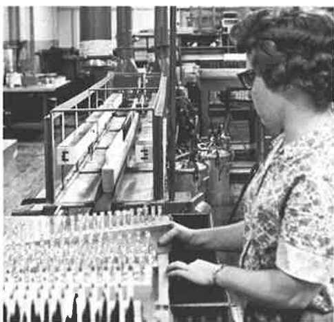
Lacquer on pen barrels must be dried quickly, also. Six units, each containing one 2500-watt quartz infrared lamp, operate under voltage; replaced PAR heat lamps for more efficiency.
