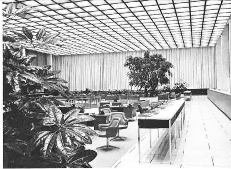
A large coffered ceiling enables a viewer to gain an impression of the size of a room — especially if he relates size of individual coffers to the size of the entire space. Lines of perspective are obvious. The edges of this lighted ceiling also tend to define the limits of the large space.
