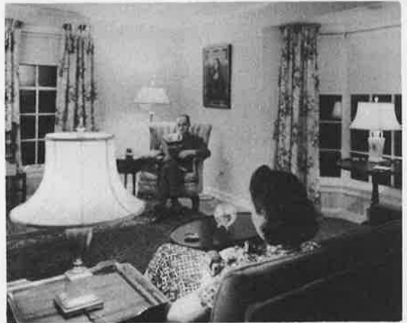
Fig. 3—Seeing conditions are greatly improved by different types of lamps, and more of them, to illuminate the surroundings, even though providing no more light on the visual task.
