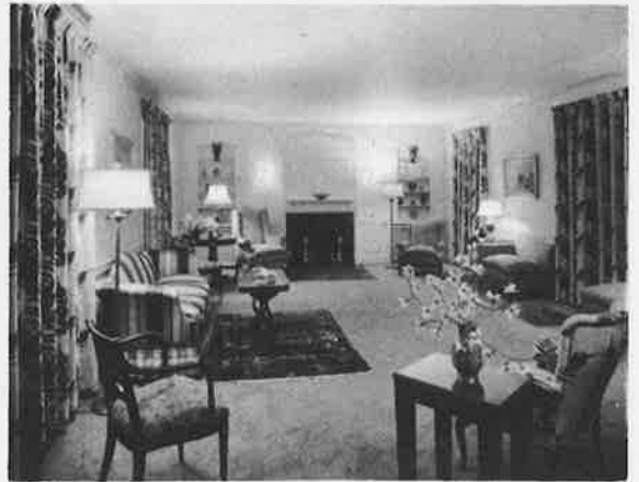
Fig. 1—In the author's living room, large areas—walls, carpet, furnishings—have relatively high reflection factor; upward and downward light is balanced; thus contrasts are subdued.
