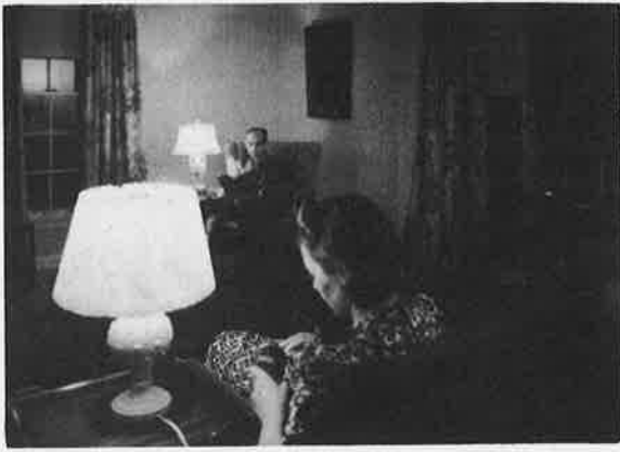
Fig. 2—Brightness-contrasts of the work (sewing or reading) and the background cause eyestrain and fatigue. This lighting may be satisfactory for conversation, but not for critical seeing.
