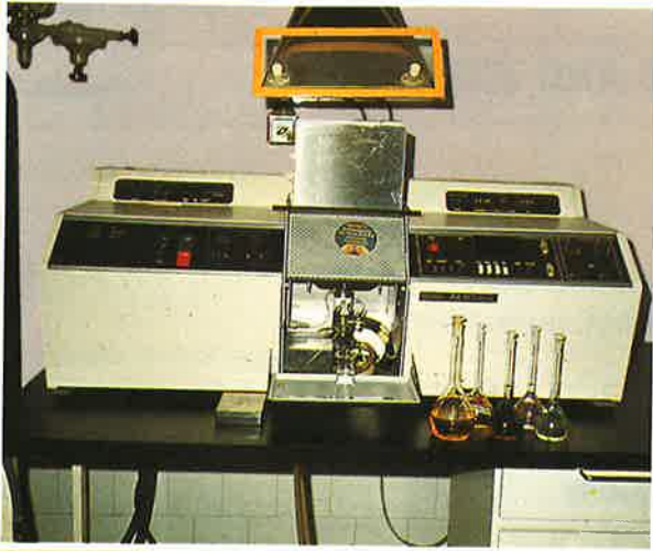
Fig. 1 Modern analytical instruments as this atomic absorption spectrophotometer shown in the photo and advanced testing methods assure the high quality of TUNGSRAM's products
