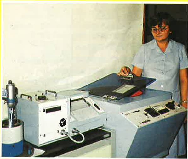
Fig. 2 Photosedimentation analyzer intended for use in determining powder particle size distributions
