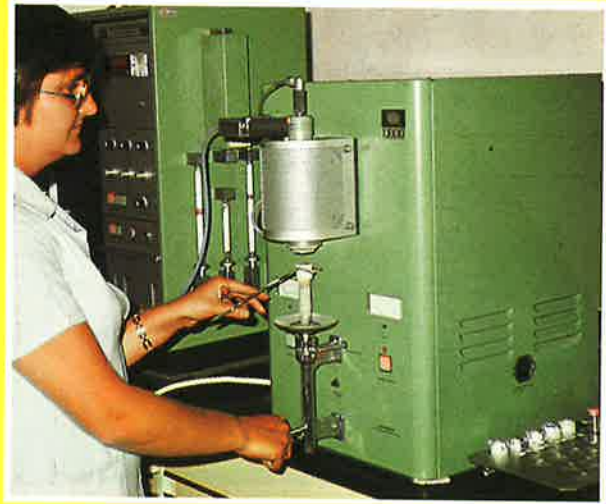
Fig. 4 Leco analyzer for carbon content test in tungsten
