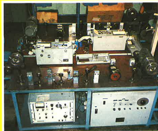
Fig. 9 Eddy current instruments test wires above 30 mg/200 for cracks and splits
