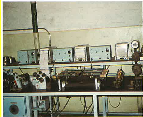
Fig. 8 Continuous diameter checking by measuring the electric resistance of wires
