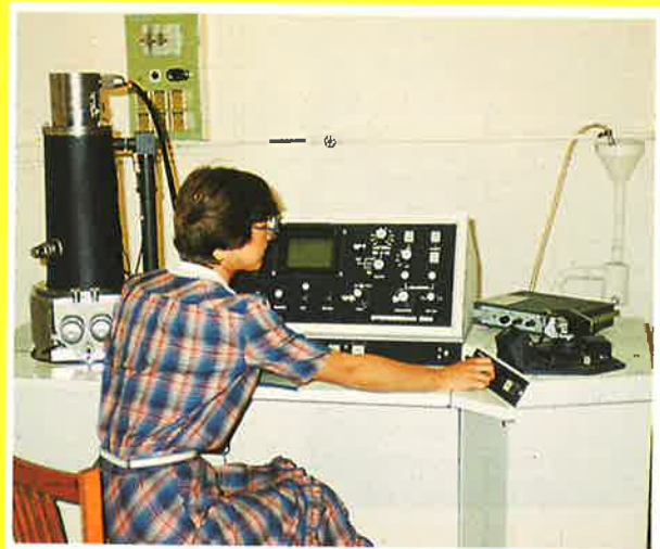
Fig. 5 Scanning electron microscope (SEM) used to test tungsten metal powders
