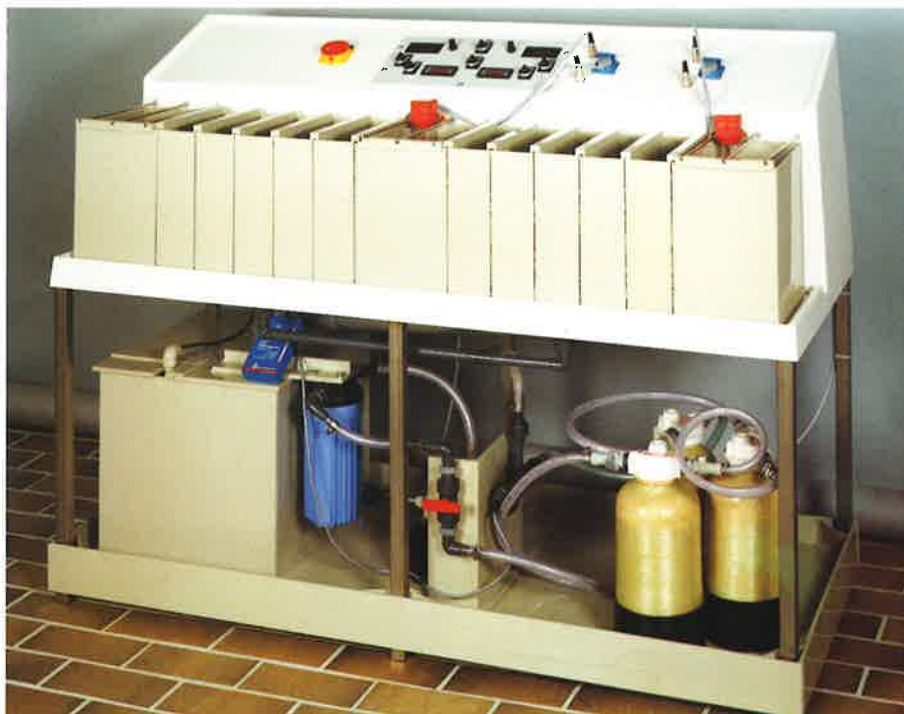
Universal electroplating unit for all conventional electroplating chemicals (with waste water re-circulation)
