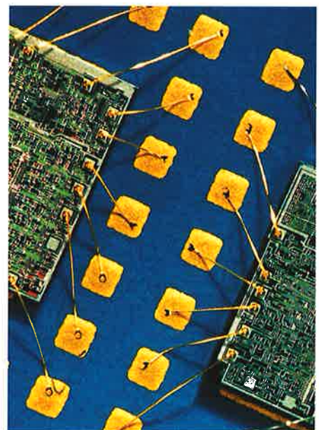
Cadmium-free gold paste G5007, bonded with 30 µm gold wire
