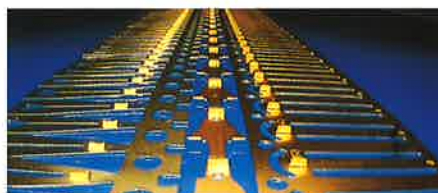
Individual welding of microcontact profile parts
