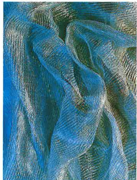
Warp knitted catalyst gauzes for ammonia oxidation to nitrogen oxides
