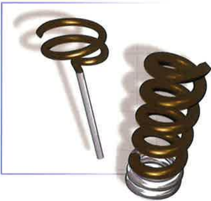
Rack coating: Cardiac pacemaker electrodes coated with TiN
