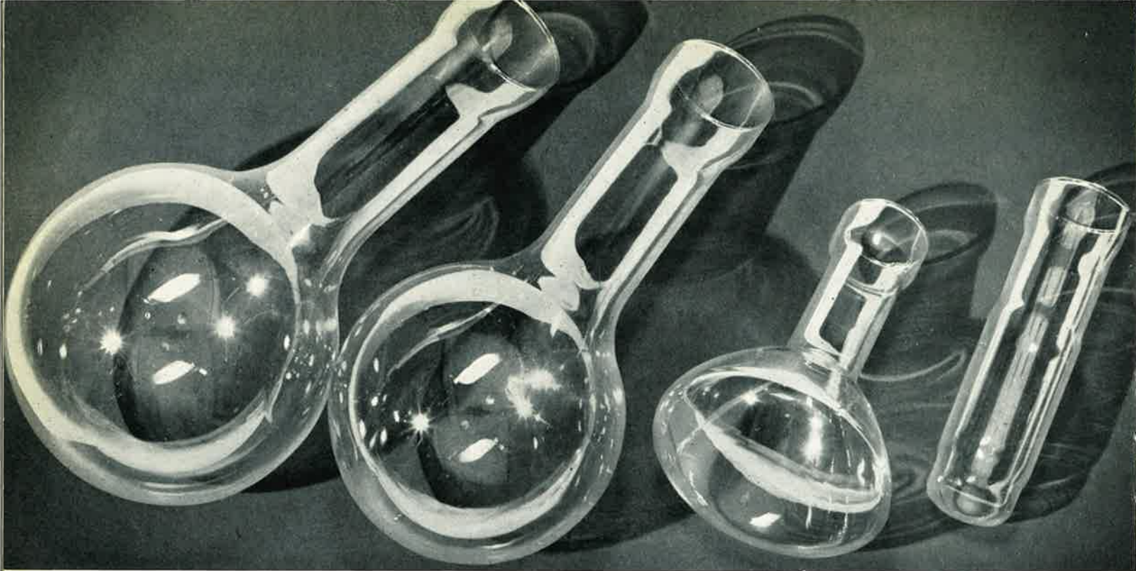
Examples of mouth-blown soda glass lamp and valve bulbs
