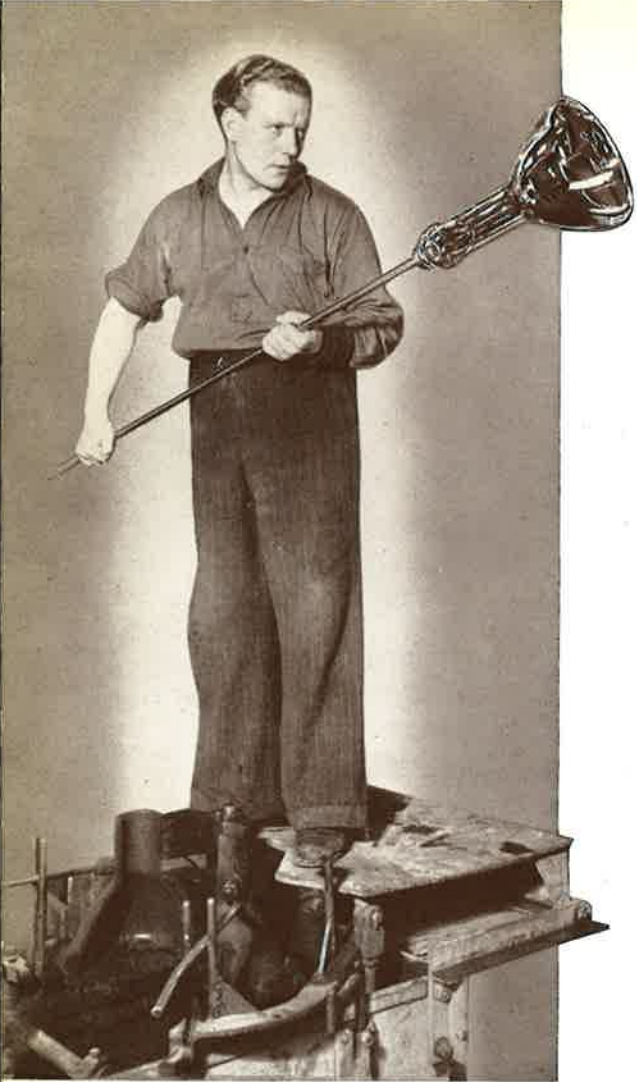
Blowing a cathode-ray tube
