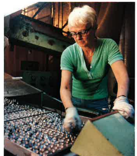
Of all our sophisticated quality control methods, one that still ranks high in reliability is the experienced eye of our inspectors. More than 5,000 parts per minute come through the inspection station shown here.
