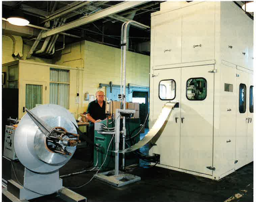
General Electric employs the latest die progression technology on presses like this 60-ton Bruderer to deep draw lamp base shells at rates of several hundred per minute.
