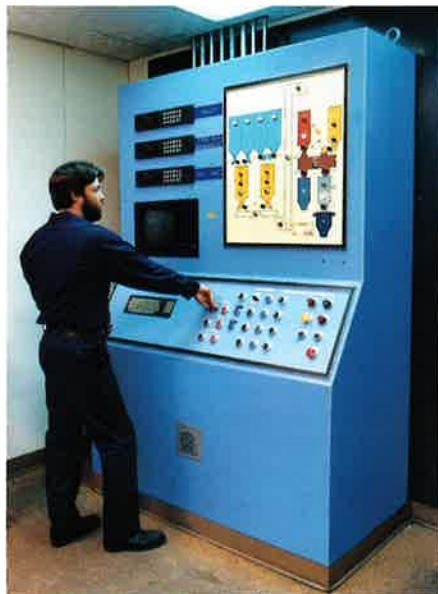
Every step in the preparation of glass for insulator sealing is controlled from this batch mixing panel, from receipt of the cullet and other constituents to delivery of the molten glass.
