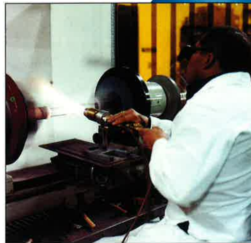
High-purity fused silica and borosilicate glassware is custom-fabricated to meet the demands of high temperature synthesis and purification of lamp materials.
