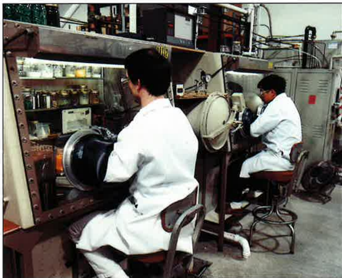
Argon-filled dry boxes maintain low parts-per-million levels of water and oxygen during the handling, sizing and ampouling of all metal halide lamp materials.
