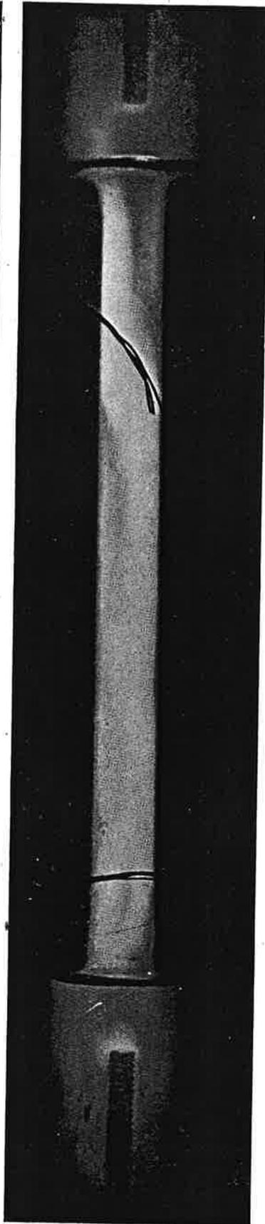
FIGURE 3 - *200-joule discharge through xenon-filled tube.*
