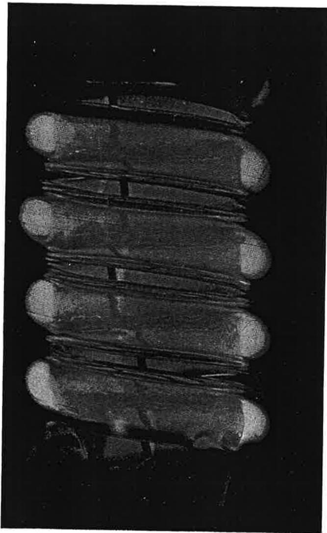
FIGURE 2 - *Helix of compact type of flash-discharge tube.*
