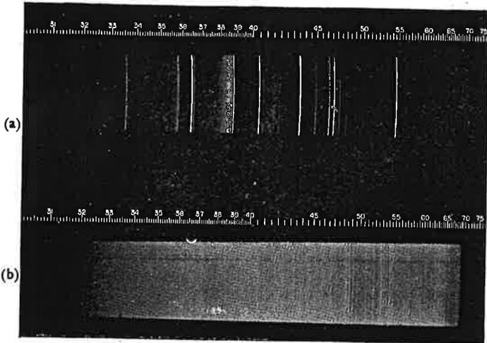
FIGURE 1 - (a) *Low-current discharge through krypton.*
