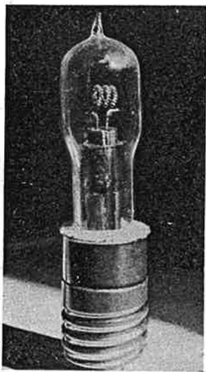
Figure 1. Experimental mercury-filled high brightness tungsten filament lamp.
