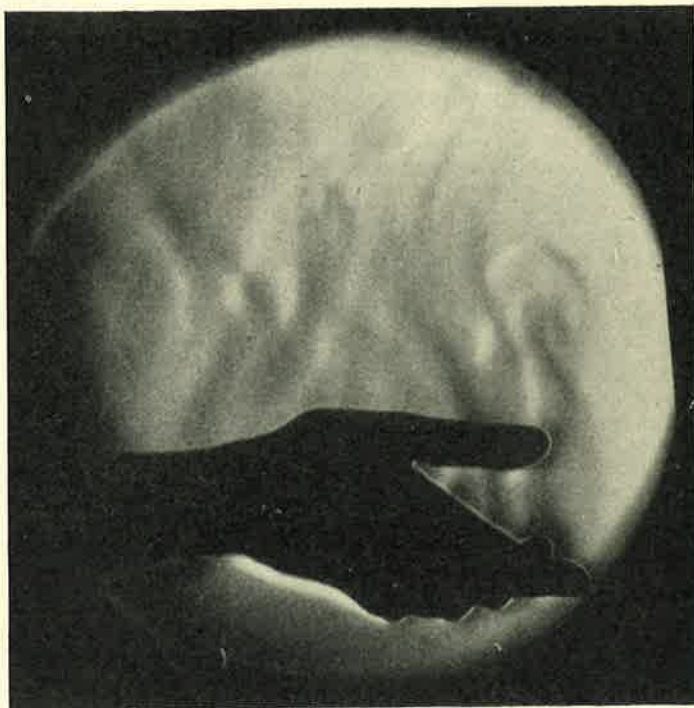
Fig. 4. Example of high-speed photography by use of the Schlieren technique, showing convection currents rising from the warmth of the hand.
