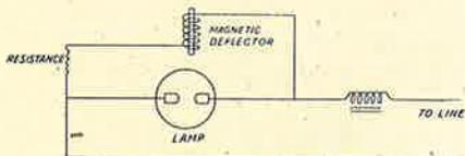
Fig. 9. Simple circuit arrangement for magnetic dispersal of arc flame.
