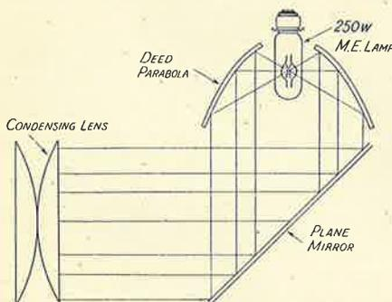
Fig. 12. Suggested arrangement of ME lamp, parabolic reflector, plane mirror and condensing lens of optical train.
