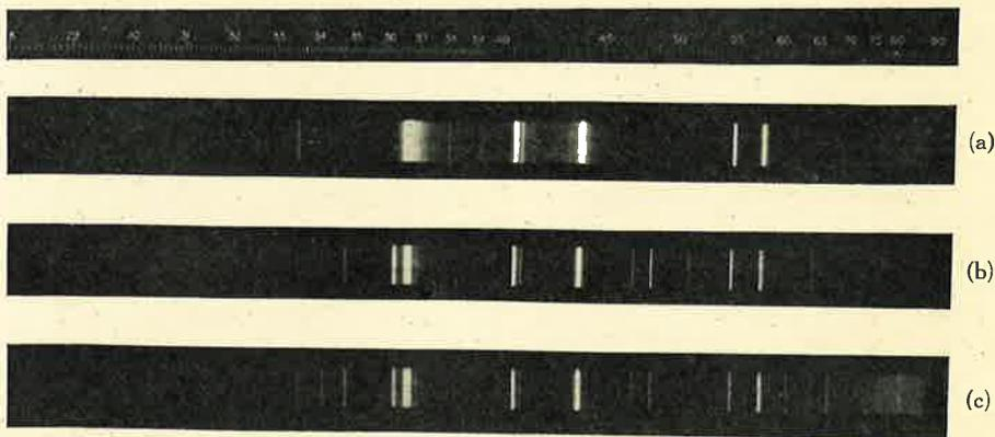
Fig. 10. Spectrograms showing radiation from mercury and mercury cadmium ME type lamps.
