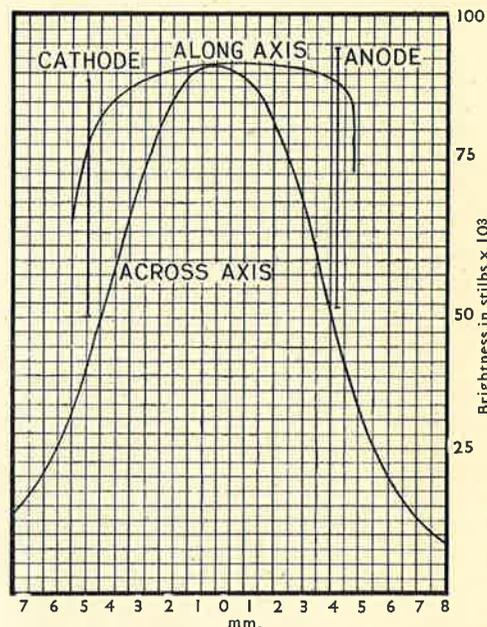
Fig. 7. Typical distribution curve for 10 kw lamp.
