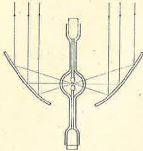
Fig. 11. Arrangement of ME lamp and deep parabolic mirror for maximum flux utilisation.
