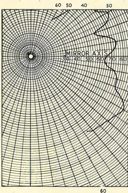
Fig. 6. Polar distribution about mirror axis of light flux from 10 kw ME lamp (wattage 10 kw, voltage 83 v., current 120 amps.).
