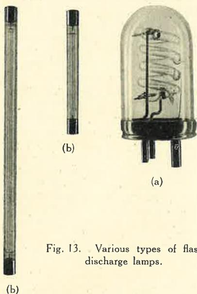
Fig. 13. Various types of flash discharge lamps.
