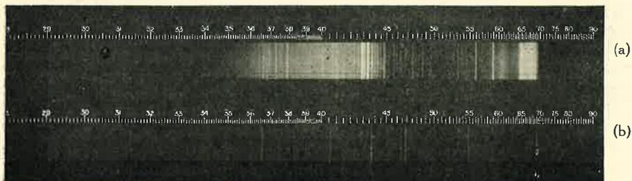
Fig. 14. Spectrogram showing discharge through Krypton-Xenon mixture.
