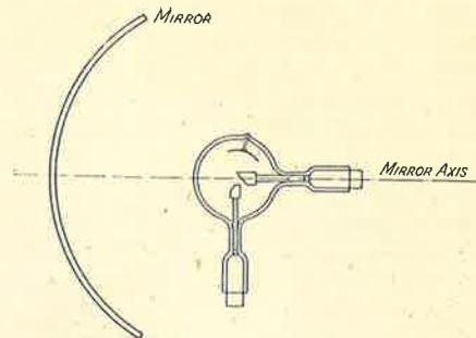
Fig. 8. Diagram of ME type lamp showing right-angle arrangement of electrodes and collector shield to intercept arc flame.
