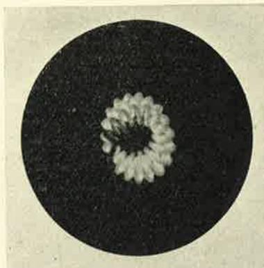
Fig. 9. End view of coiled coil filament in operation, showing end cooling effects and effect of internal reflections.
