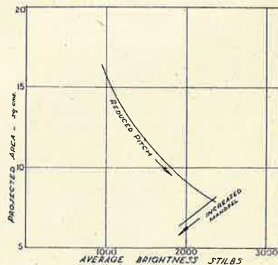
Fig. 15. Variation of brightness with area, for 12-volt, 72-watt filaments operating at 21 L/w.; consisting of two 12-volt, 36-watt coils in parallel.
