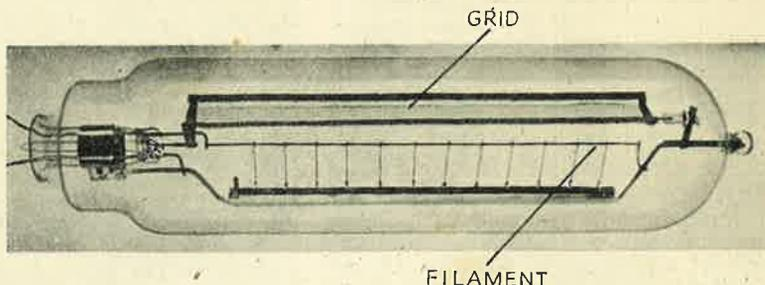
designed specifically for use with optical projection systems where, in general, sources of small size and the highest possible brightness are required.
