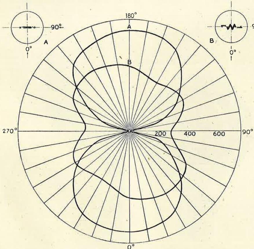
Fig. 13. Candlepower distribution for 12-volt, 200-watt lamps. A, solid source. B, coiled coil.
