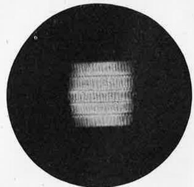
Fig. 12. Filament of 12-volt, 300-watt "solid source" lamp in operation.
