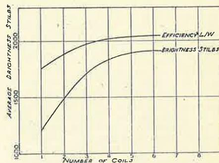
Fig 14. Variation of average filament brightness with number of filament coils arranged in solid source formation.
