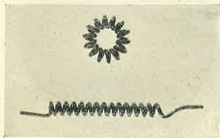
Fig. 8. Primary coil before and after bending into coiled coil formation.
