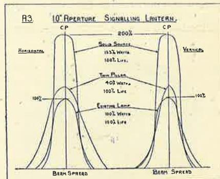
RELATIVE PERFORMANCE OF HIGH PRECISION SIGNALLING LANTERNS WITH EXISTING LAMPS AND WITH CERTAIN OF THE LAMPS DESCRIBED IN THIS PAPER.
