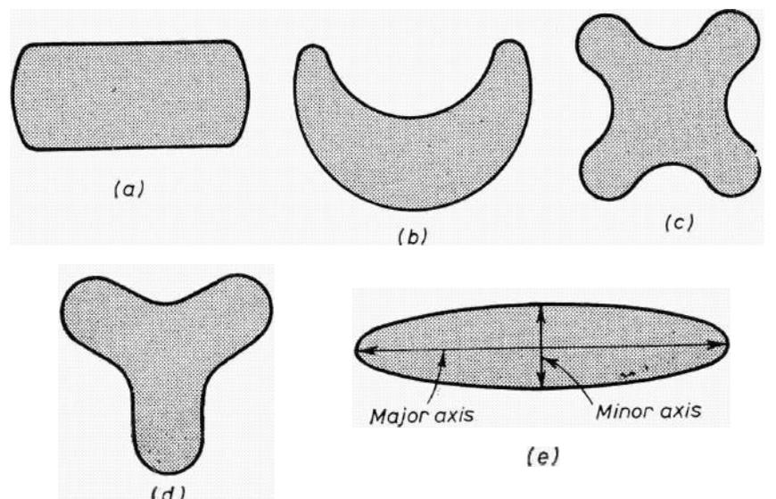
Fig. 4. Various possible cross-sectional shapes for high efficiency sodium lamp arc tubes
