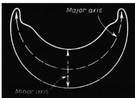
**Fig. 5. The crescent-shape cross section finally developed for the new AEL linear arc tube sodium lamp. Liquid metal resides in the regions of smallest radius by virtue of capillary action**
