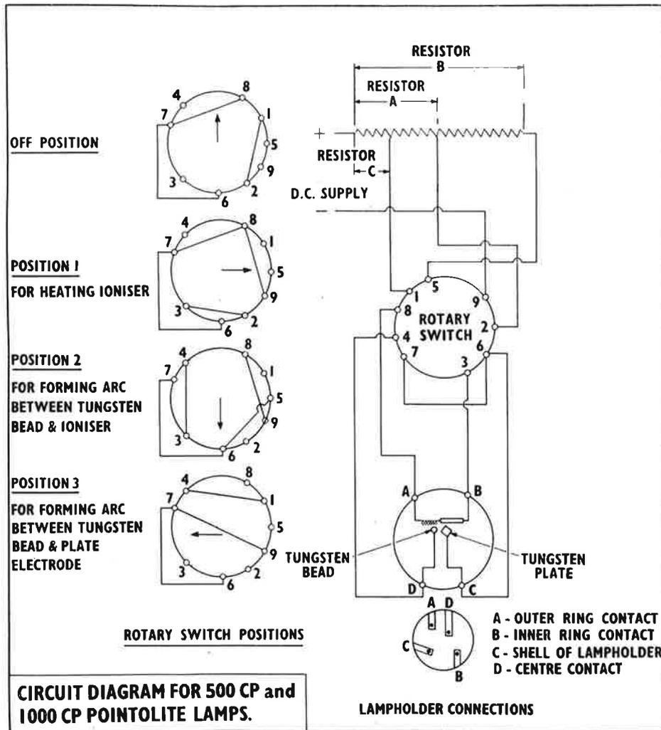
The Rotary Switch shown in the above diagram must be of the rapid action type, as it is imperative that the change from position 2 to position 3 be made instantaneously.
