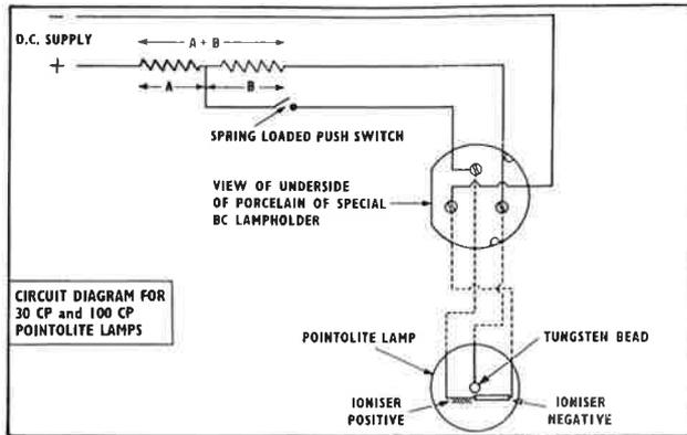
The special three plunger lampholder requires to be wired with three core flexible cable, and it is imperative that the wiring of the lampholder is as shown above.
