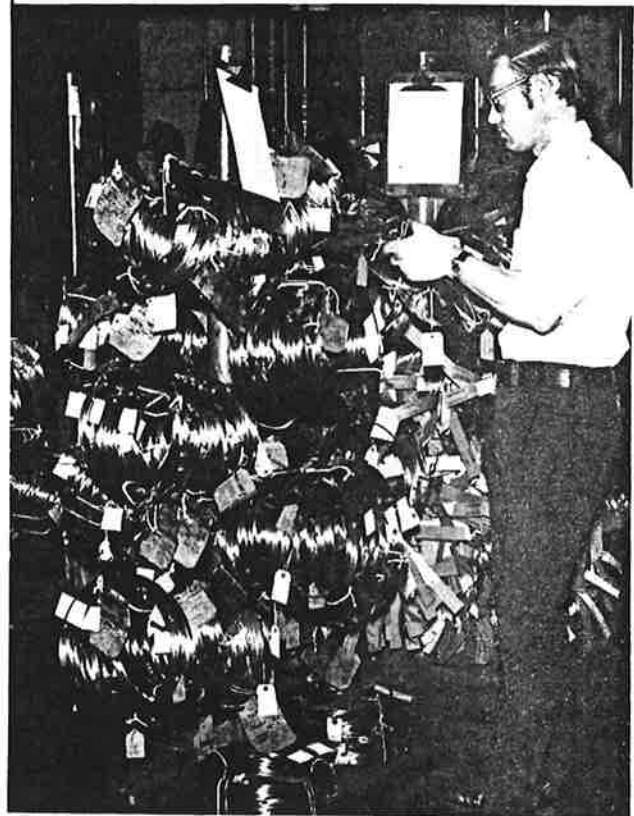
Heavy tungsten wire ready for further drawing
