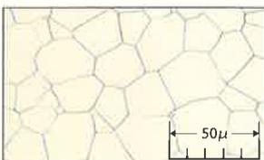
Polycrystalline sintered to high density (HICERAM thermally etched surface)
