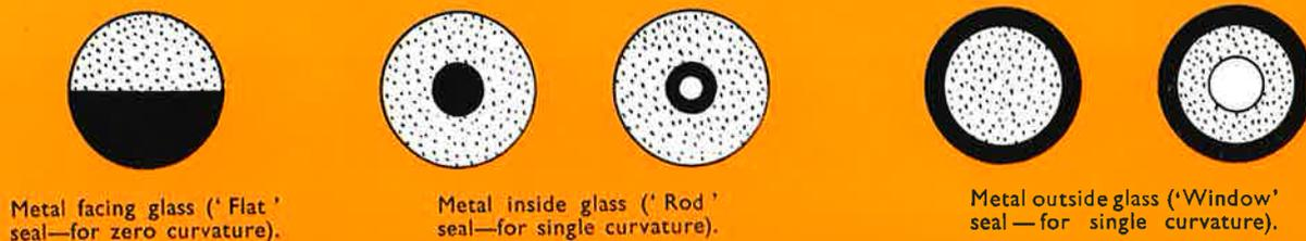
Fig. 2.—Diagram showing the three basic types of seals. (By courtesy of The British Thomson-Houston Co. Ltd.)
