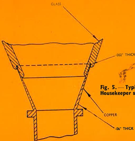
Fig. 5.— Typical Housekeeper seal.
