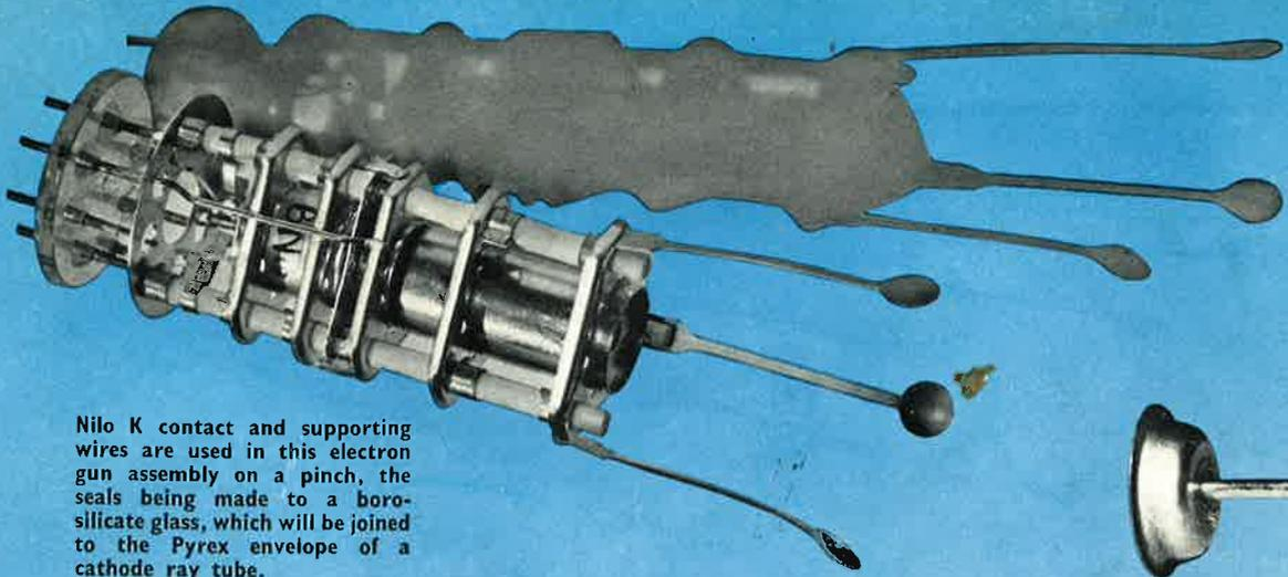
Nilo K contact and supporting wires are used in this electron gun assembly on a pinch, the seals being made to a borosilicate glass, which will be joined to the Pyrex envelope of a cathode ray tube.
