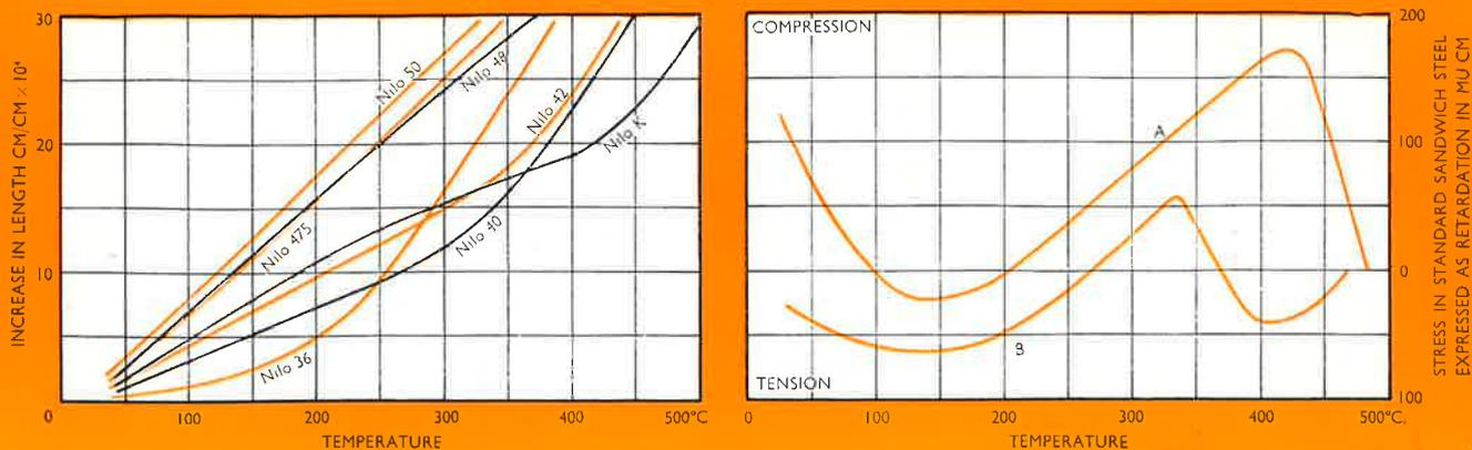
Fig. 7.—The curves on the left show the thermal expansion of the iron-nickel alloys of the Nilo series in the fully annealed condition. On the right are shown the stress—temperature curves for Nilo K with C.40 glass (A) and Nilo 475 with C.12 (B) glass.
