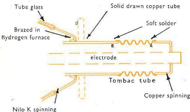
D. Supporting ring to support the flex tube when under vacuum conditions
