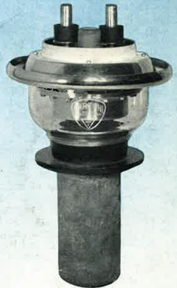
Two types of wireless transmitting valve in which Nilo K is used for the glass-metal seal.
