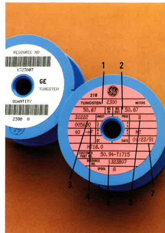
**Computer generated labels (right) have the wire processing information that confirms the finished wire specifications. Bar coding (left) is used to speed order processing and maintain good inventory control.**
