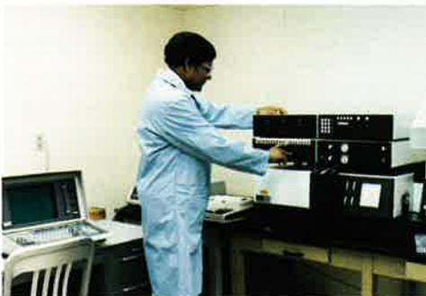
On the direct coupled plasma spectrometer (DCP), up to 19 elements in solution can be identified and measured simultaneously.
