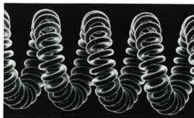
The inset shows a greatly magnified view of a coiled coil tungsten lamp filament.
