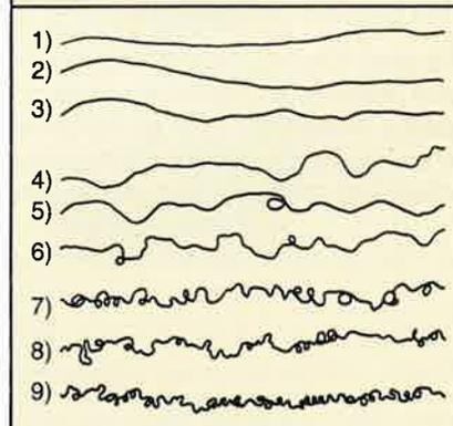
In determining degree of curl, a two-foot length of wire is allowed to hang in a 1" catenary. It is then compared to this chart and rated accordingly.
