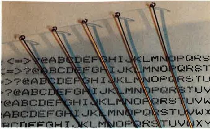
An array of tungsten metallizing coils.
