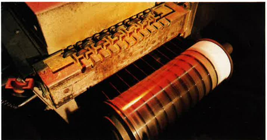
Multiple die equipment in which temperature, drawing speed, and die geometry are carefully controlled, is used to produce very small diameter tungsten wire.
