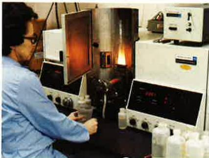
The elevated temperature strength properties are measured to better understand the response of wire to varying application conditions. Wire is normally tested in hydrogen although it can be measured in either vacuum or inert atmospheres.
