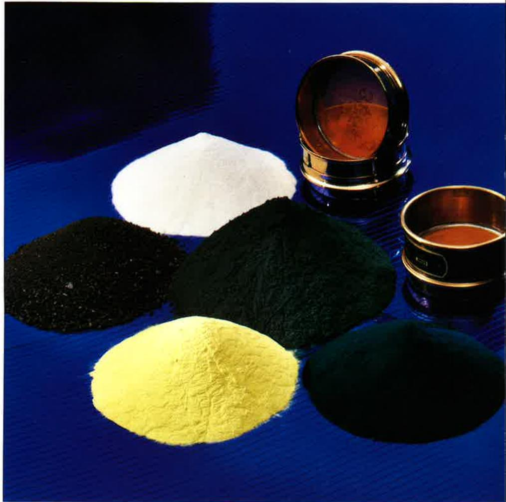
Tungsten powder is produced by the hydrogen reduction of an oxide. Powders are a mixture of semi-sintered aggregates of small basic particles.
