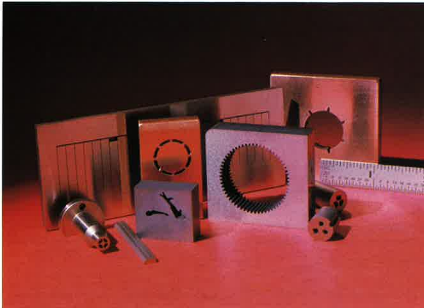
This array of parts was produced by electrical discharge machining using molybdenum wire as the cutting tool.
