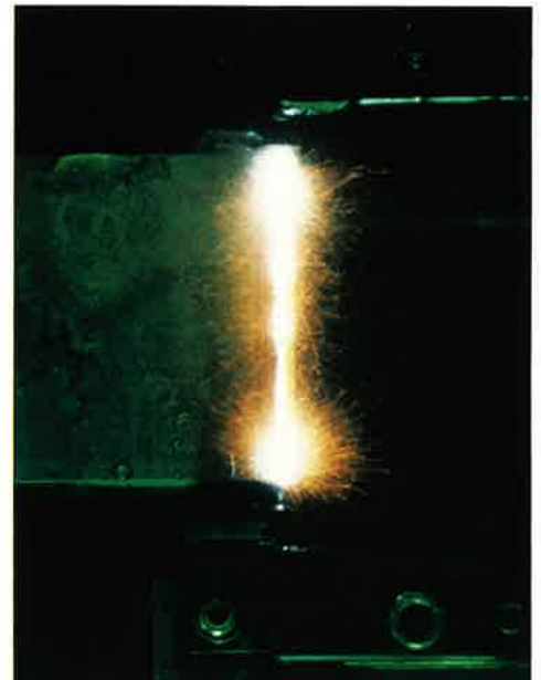
In operation, the molybdenum wire maintains sufficient strength at high temperatures under adverse conditions to provide precise cuts in carbide, steel, copper and other materials.
