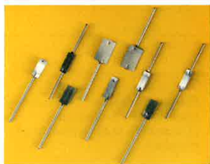
For many quartz or hard glass seals, etched foil lead assemblies utilize tabs of platinum clad ribbon to create an effective weld joint between the foil and lead wire.
