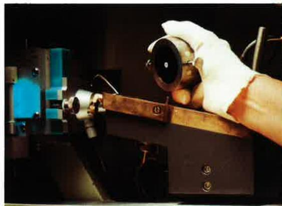
*The chemistry on each heat of core rod is verified for conformance to specification.*
