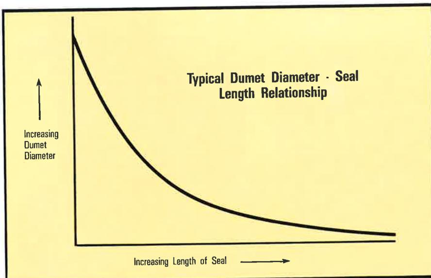
Figure 2 - Diameter/Seal Length Relationships
