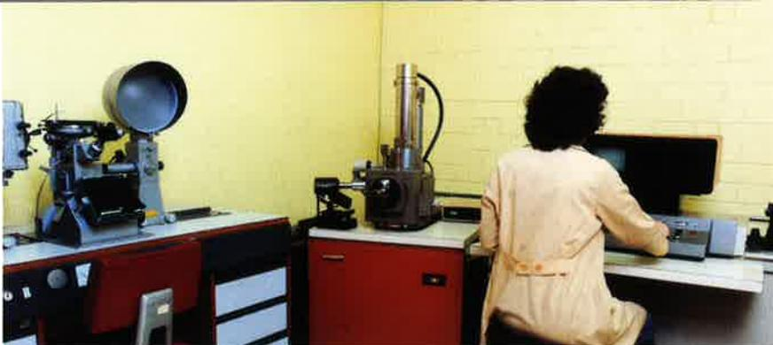
*GE uses a number of test instruments to look for possible defects in the oxidized or coated surface.*
