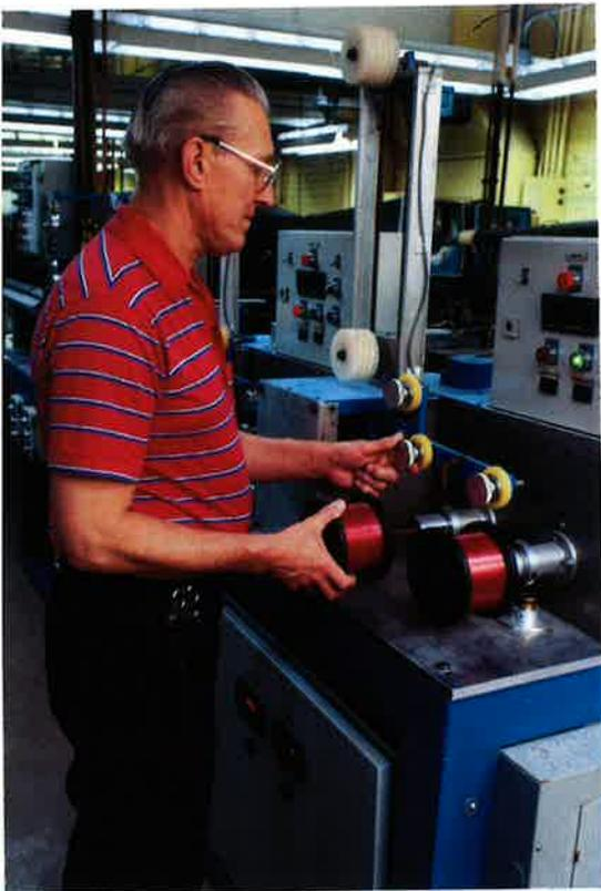
*A new borating line at GE's Carolina Welds plant features power assisted payoff, preoxidation burners, acid clean and rinse cycles, atmospheric cooling tubes, and tension reels to control the wire speed through the heating zones and borate quench tank.*
