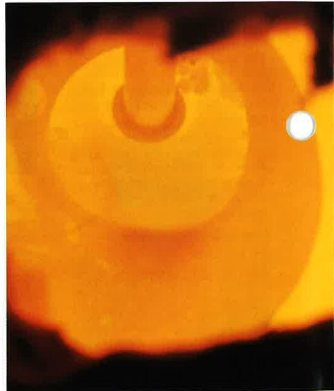
*In the crucible, copper is metallurgically bonded to the core rod.*
