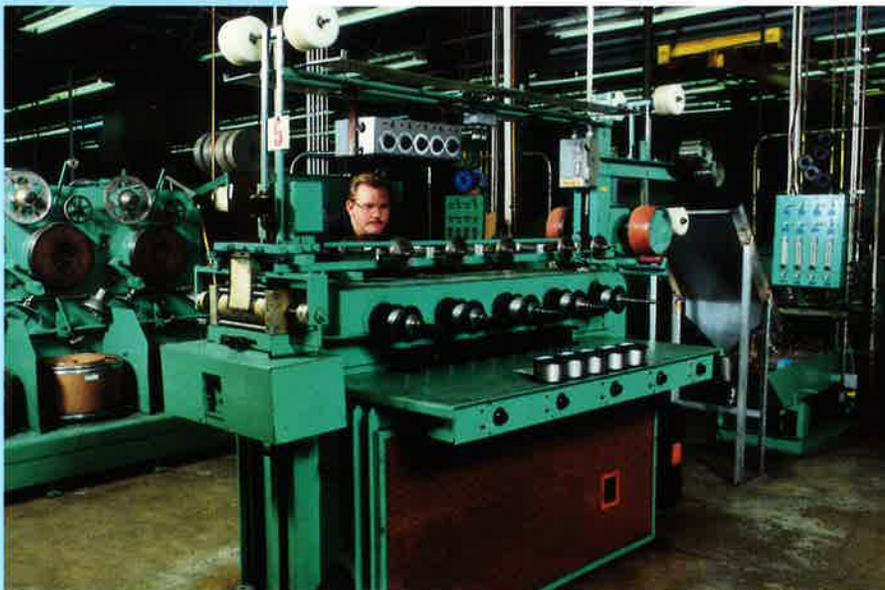
*Wire is kept under tension through the annealing furnace so its speed can be carefully controlled. This enables operators to achieve more exact properties in the final product.*
