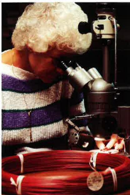
*Before GE wire is shipped to the customer, it is thoroughly analyzed for surface defects.*
