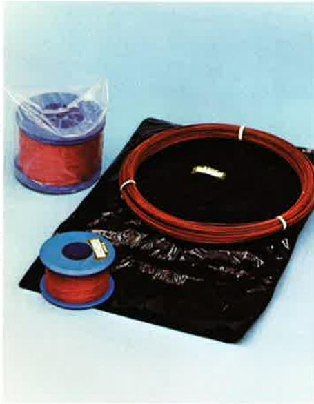
Dumet wire in the range of 10 to 30 mil diameters is shipped on either 5 or 10-pound spools contained in clear heat-sealed plastic bags with a desiccant. In the 30 to 125 mil range, Dumet is wound into 10-pound self-contained coils that are tied and shipped in sealed black plastic bags with a desiccant.
