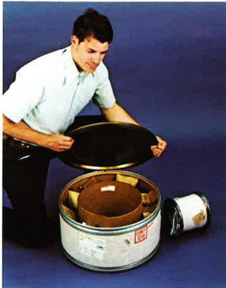
Cumet is available in 80 to 100-pound pail packs or on 30-pound spools. The pail packs are flat drums in which the wire is wound around a central core so that it can be continuously fed from the pail to automatic processing or assembly machinery.
