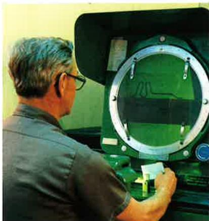
*On the comparator, intricate formed wire parts are visually inspected at several times actual size to detect any dimensional variations that may be occurring because of tool wear or other small changes in the processing equipment.*
