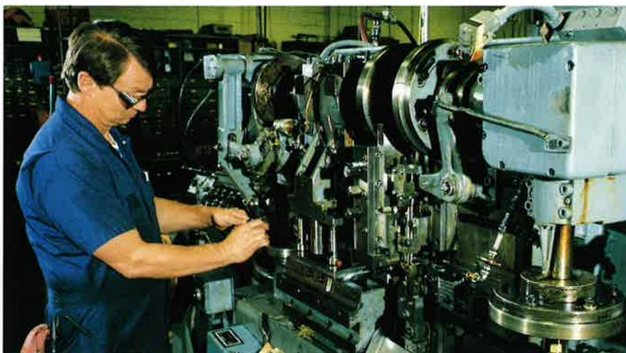
*High quality parts featuring multiple bends and intricate cuts are processed at high speeds on this verti-slide forming press. It handles a full range of materials, from soft brass to molybdenum ribbon.*
