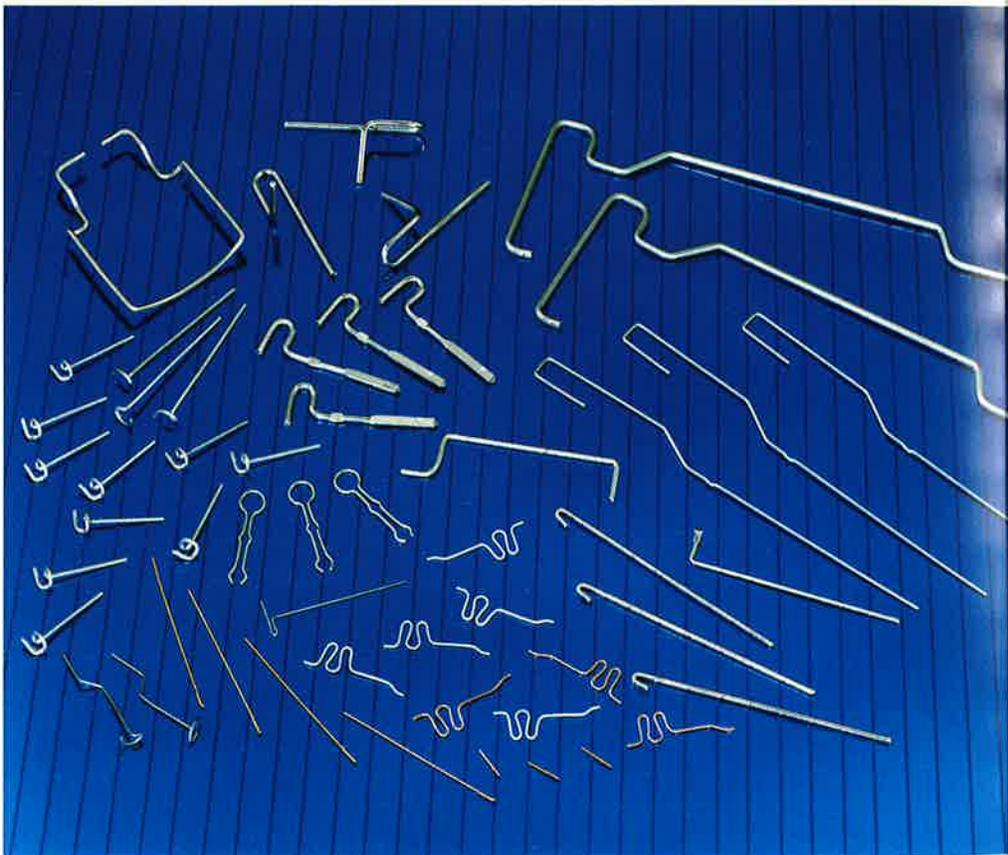
*The complex workings of this high speed multi-slide press turn out between 300 and 600 multiple bend parts every minute. Starting materials cover a range from very thin wire gauges to one inch wide ribbon.*
