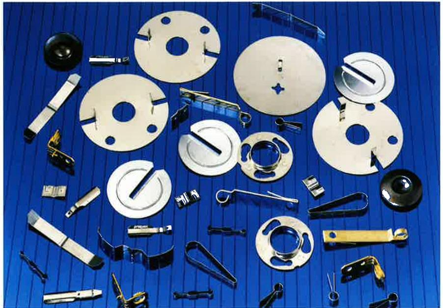
*Forming thin gauge metals takes a light touch. Many of these parts require plating or blanking before press operations.*
