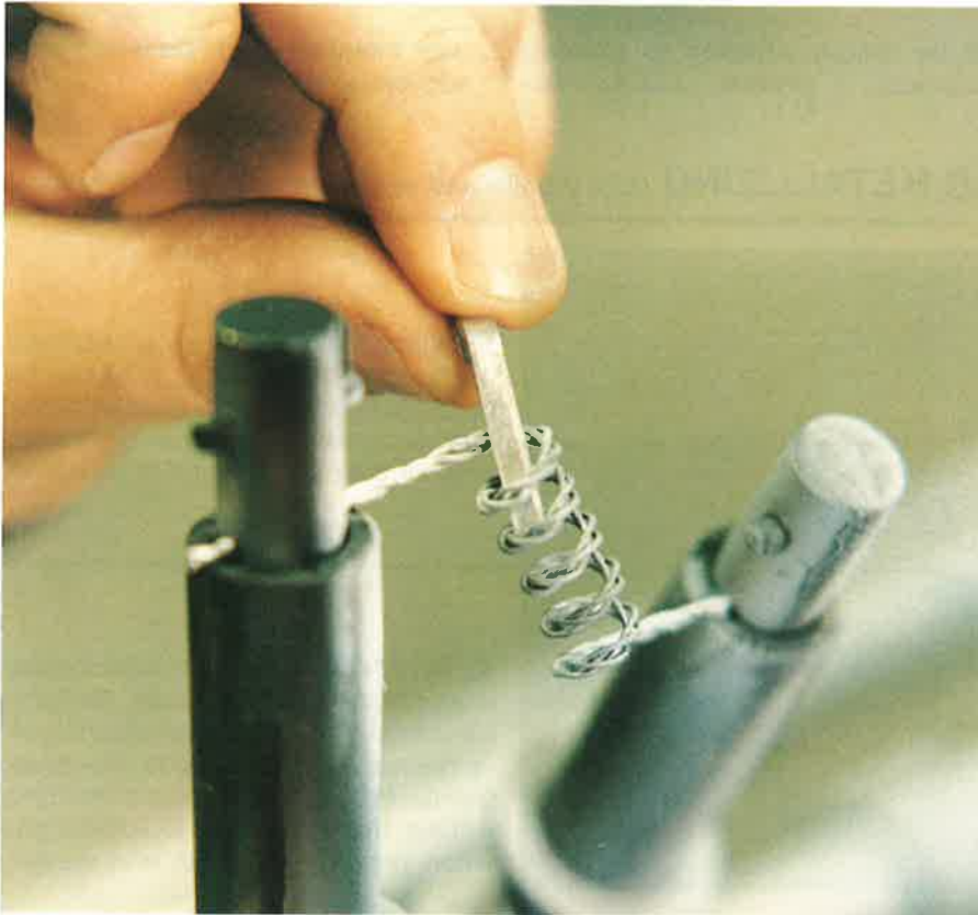
Loading of the vertical coil is done by dropping an aluminum cane into the coil body, a much faster operation than pinching on small clips. A special modification of electrode posts is needed for using vertical coils, as indicated in the right hand photo.
