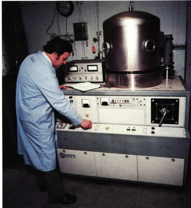
Simulated life and coating tests are run in this vacuum bell jar to generate the data which enables General Electric engineers to design coils for a variety of metallizing applications.
