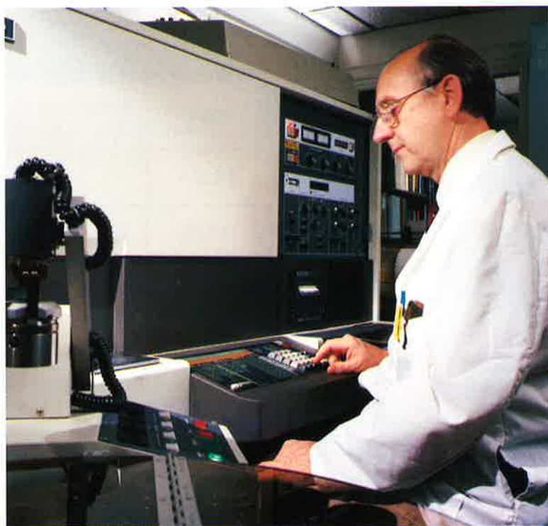
Quantitative and qualitative analysis of fused quartz constituents is provided by X-ray fluorescence (above) and other instrumentation.
