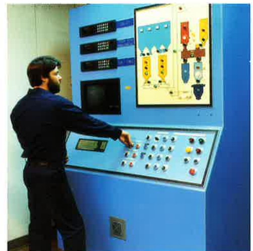
Every step in the preparation of glass for sealing is controlled from this batch mixing panel, from receipt of the cullet and other constituents to delivery of the molten glass.
