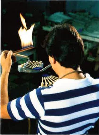
Glass tubing containing 20 to 30% lead is workable at low temperatures, permitting neon sign artisans to form the material into intricate shapes.
