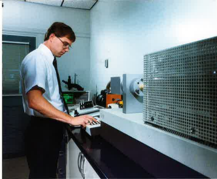
The tendency of the glass to expand and contract at different rates is studied on the dilatometer in our materials characterization laboratory. Machined samples are placed in vacuum or atmosphere, and dimensional changes are recorded automatically as the temperature is increased to the material's softening point.
