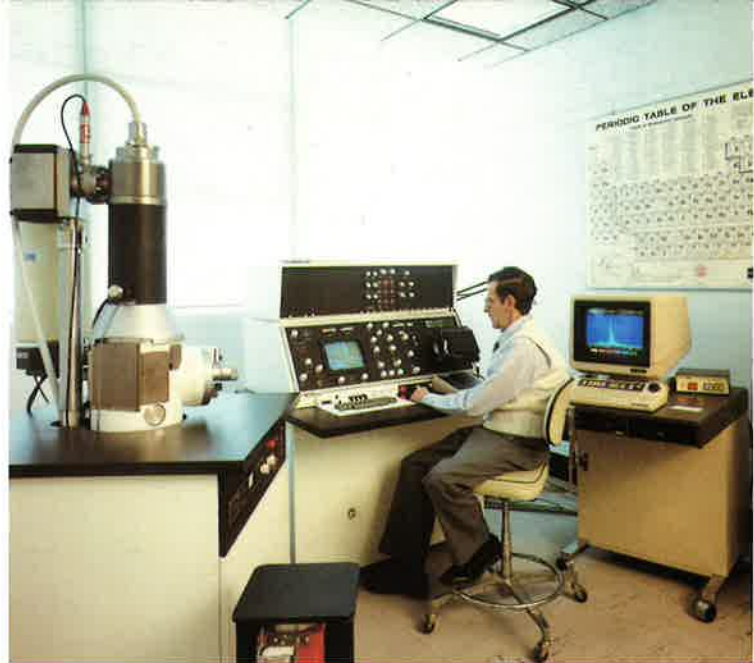
On our scanning electron microscope, the microstructures of such materials as tungsten, molybdenum and phosphors are studied at magnifications of up to 10,000 times.
