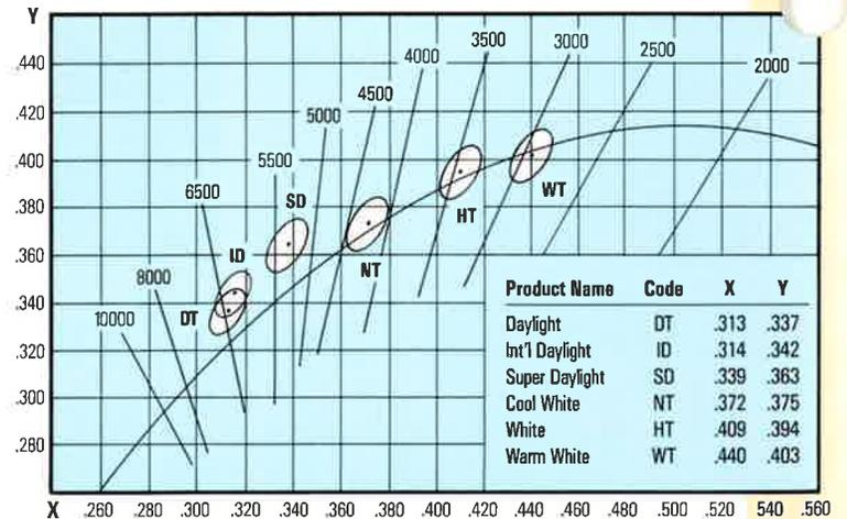
This schematic diagram provides a visual profile of the color characteristics of several GE phosphors. They show the radiant power emitted by the source at each wavelength or band of wavelengths over the visible region (360 to 720nm).
