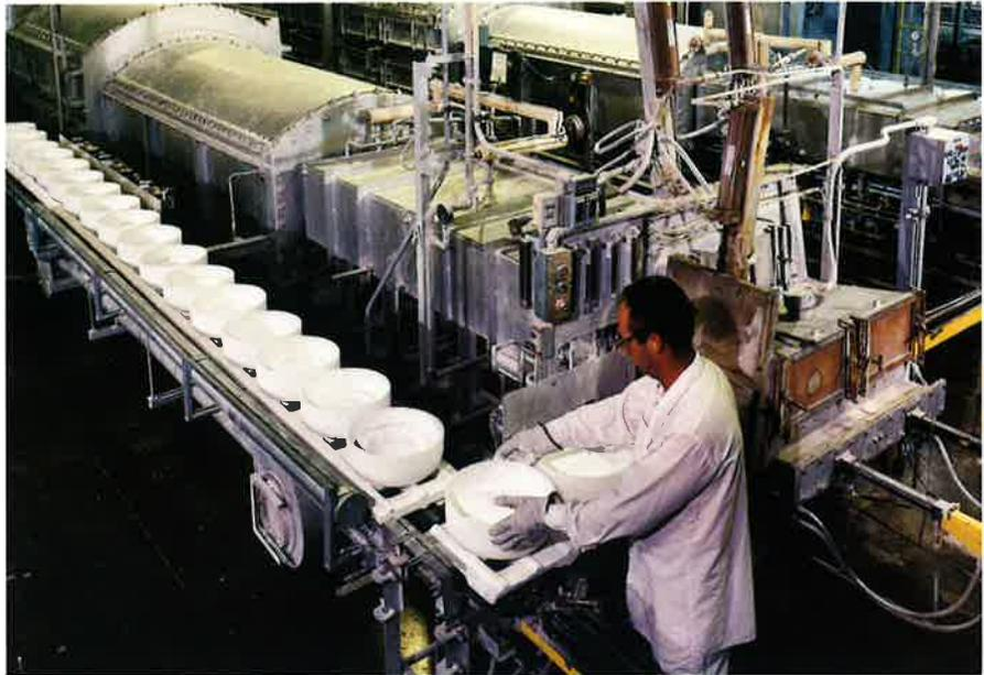
*This tunnel furnace provides the controlled firing conditions required for maximum brightness and particle size control of lamp phosphors.*
