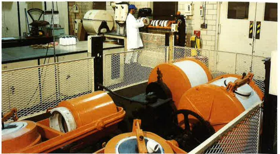
*A variety of specialized equipment is used for controlled size reduction. Precision ball mills shown here, Trost, Bauer, ACM and others, reduce particle size to submicron levels and also adjust the surface area of the particles to achieve the desired chemical reactivity.*
