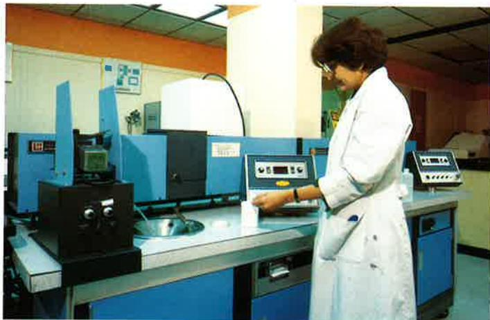
*A statistical analysis of the particle size distribution of a chemical is summarized and printed out for study on this Leeds & Northrup Microtrac small particle analyzer.*
