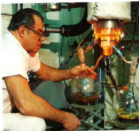
*Although our primary products are inorganic chemicals, GE also produces specialty solvents, organic dyes, and a low molecular weight polymer. In the high vacuum distillation process, shown here, low molecular weight polymers are separated in a molecular still.*
