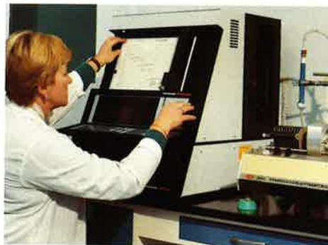
*The physical characteristics of chemicals are studied on the thermogravimetric equipment shown here, as well as on our X-ray diffraction and differential thermal analysis apparatus.*
