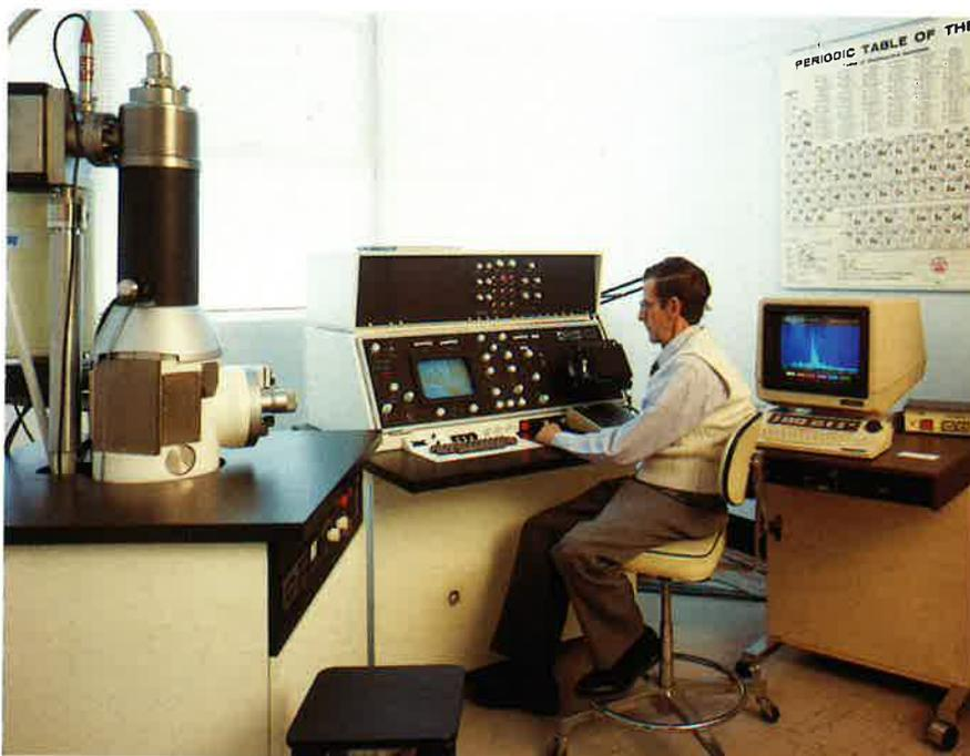
*On the scanning electron microscope, size, distribution, shape and morphology of crystals are viewed and studied. At magnifications up to 100,000 X, it is possible to study submicron sizes. Among the other particle size measurements we provide are Coulter Counter, Fisher Sub Sieve Sizer and Cilas Granulometer.*
