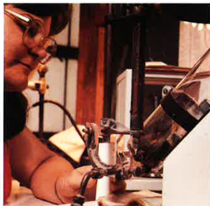
Spraying loose filaments in a sealed chamber as they are agitated by air pressure provides a uniformly thin coating of getter over the entire surface.
