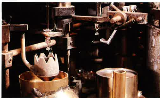
Most getting is on the same high production machines where the bulb stem is produced. Here, a cup of getter is raised from its tank to cover a filament. Next in line, an applicator dips into lead getter and gently dabs the lead wires of the completed stem.
