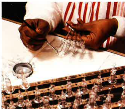
For short run situations or stem shapes that cannot be adapted for mass production, lead wire getters are painted on by hand.
