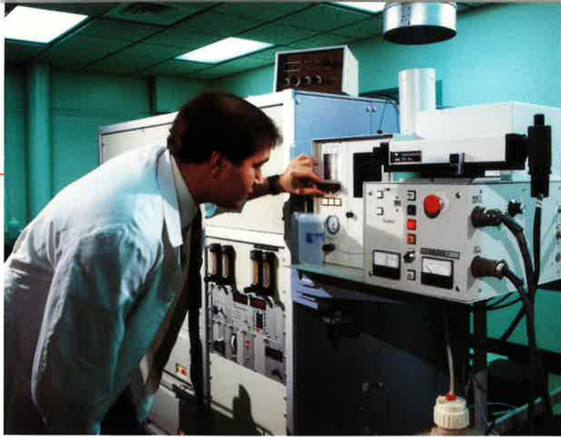
Inductively coupled plasma spectrometer is used to analyze impurities in tungsten, from ore to finished product.
