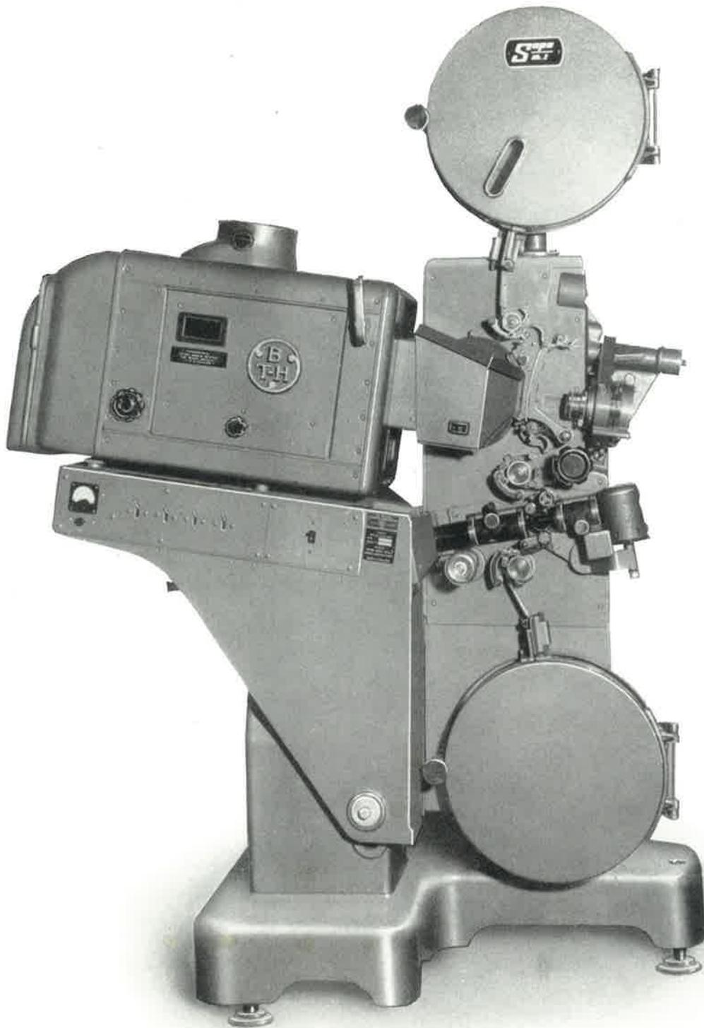
Fig. 1. BTH Supa Mark 2 projection equipment, with Type LX xenon-lamp lantern.
