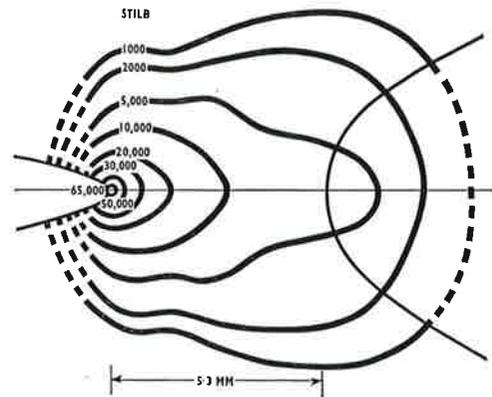
Fig. 7. Brightness distribution for similar lamp with 5.3 mm. arc gap.
