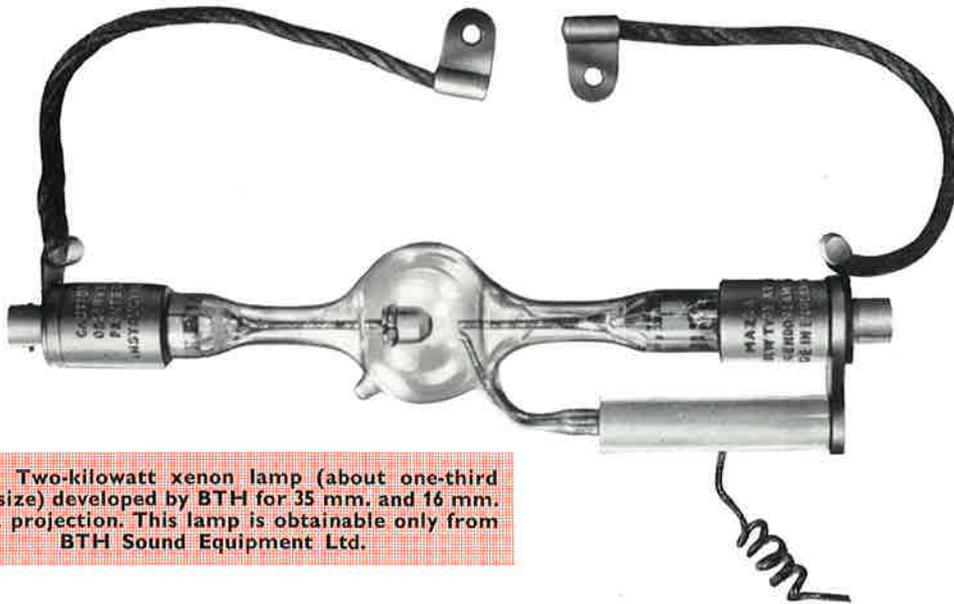
**Fig. 2. Two-kilowatt xenon lamp (about one-third actual size) developed by BTH for 35 mm. and 16 mm. cinema projection. This lamp is obtainable only from BTH Sound Equipment Ltd.**
